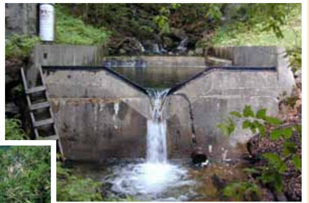
Figure 27. Weir for measuring stream flow. Copyright Hubbard Brook Experimental Forest. Source: USDA, www.hubbardbrook.org
