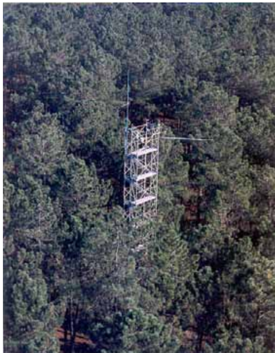
Figure 19. Eddy flux tower for assessing gas (water vapour, CO 2 ) exchanges between a Pinus pinaster forest and atmosphere in Portugal. Photo by J. Soares David.
