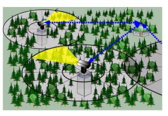
different technic and human resources to manage them. Special focus on the **FIREWATCH** vigilance system: 84 automatic towers with optical sensors (OSS) that send information to 25 offices.
