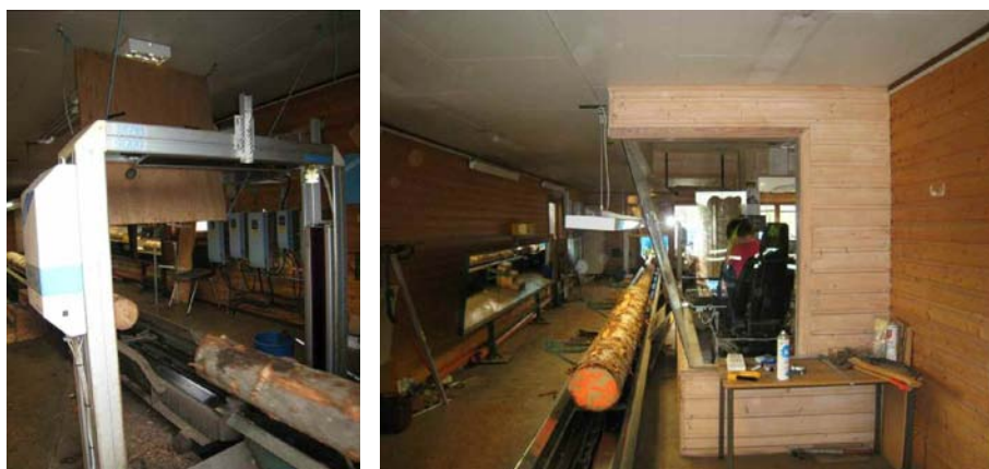
Figure 4: Sawlog scaling in log scanner at industrial sawmill (left); quality grading is done by visual assessment while logs are moved by a conveyor
