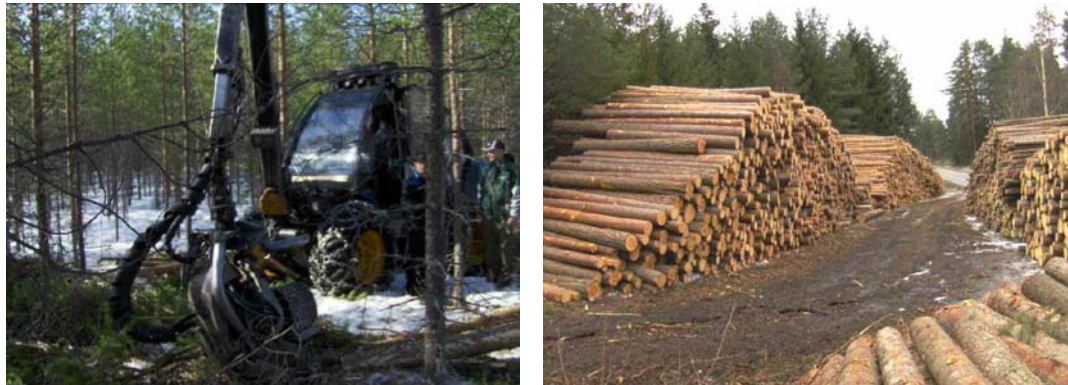
Figure 3: Cutting – both thinning and clear-cutting – is highly mechanised and computerised to optimise bucking (left); forest owners deliver their logs at roadside, separated in assortments e.g. pine sawlogs (right).
